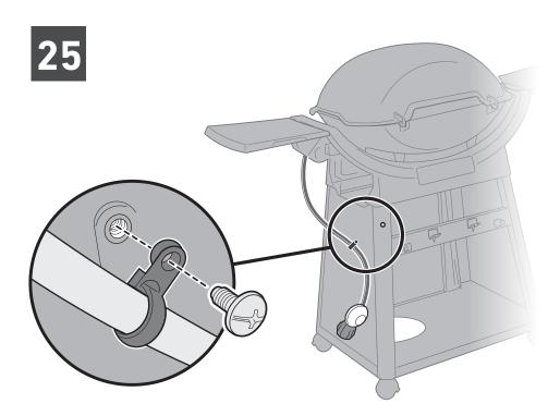
Remove screw and secure hose and retention clip to cart.
