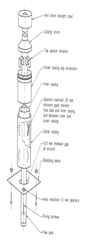
WARNING: The Fire and Flue System shall be installed in accordance with AS/NZS 2918:2001 Appendix F and the appropriate requirements of the relevant building code or codes. Firenzo/SFP Flue Kits or Davin Flue Kits must be used.
