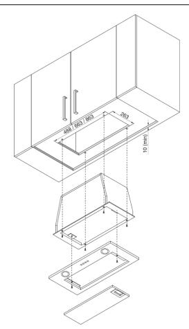
Install Range Hoods in accordance with the manufacturer's instructions. Technika recommends that all Range Hood clearances be a minimum of 650mm to a maximum of 750mm (between the top of the cooking surface and to the underside of the rangehood).
