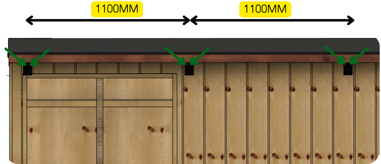
BARN DOOR BRACKETS INSTALLED 1100MM APART
