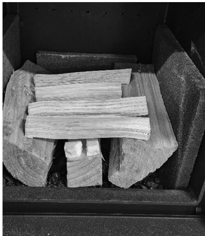
Step 1 - Building the fire – Air control full open (high). Place large sized pieces of fuel in the base and build a kindling cross stack on top
