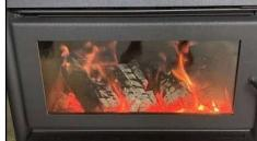
**STEP 6** – The door should be kept shut until the fuel is well burnt down until glowing embers with small flames of about 6 cm high are present in the base of the fire.
