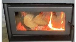
**STEP 8** –Once the fire is well established then the air control can be adjusted to lower heat settings.
