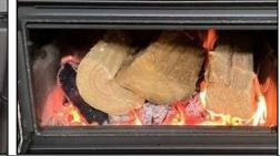
STEP 7 – Crack the door open and wait 5-10 seconds. Then slowly open the door. Place seasoned large logs on the ember bed and shut the door. Carry out the reloading in a minimal amount of time so as not to allow the flue temperature to drop too much.
