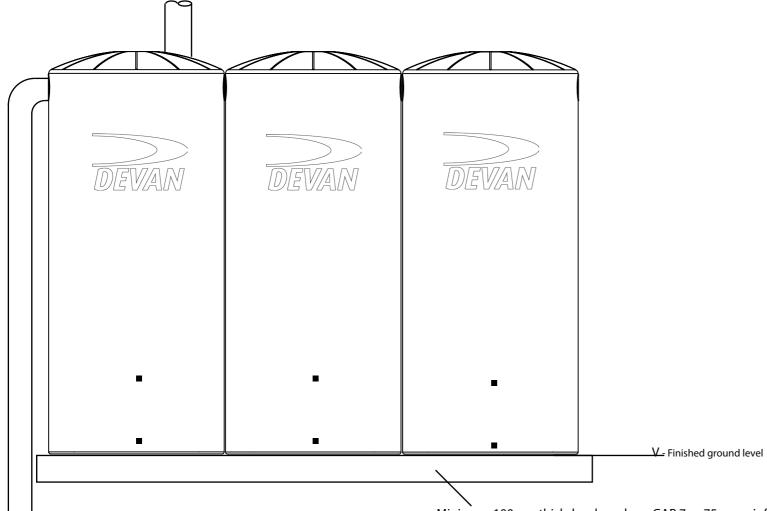
Minimum 100mm thick, level sand or <GAP 7 or 75mm reinforced concrete slab. 150mm wider and longer than over all width and length of tanks
