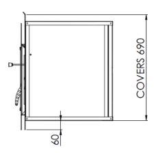
When using the Standard Topaz Fascia, the base of the fire must be elevated a minimum of 200mm above the hearth surface. An Ash Floor Protector may be used.
