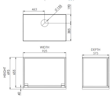
Note: The Zero Clearance Box includes a 40mm non-combustible base
