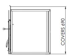
When installing the fire flush with the hearth surface, the Topaz Lowline Fascia must be used.
