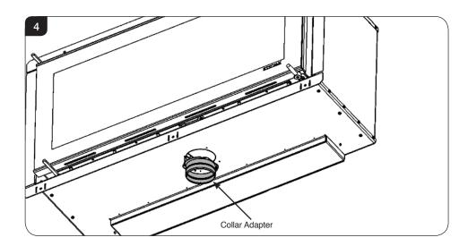
4a.3 Fix hose to collar adapter and secure duct with fixing band, see Diagram 5.
