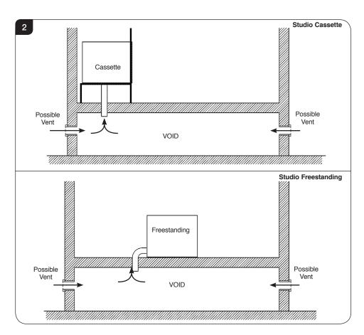
3.3 Terminations should be made with a proprietary fixed open external air vent kit, which gives minimum free area of greater than listed, positioned so no blockage can occur and not permit the entry of birds or animals.
